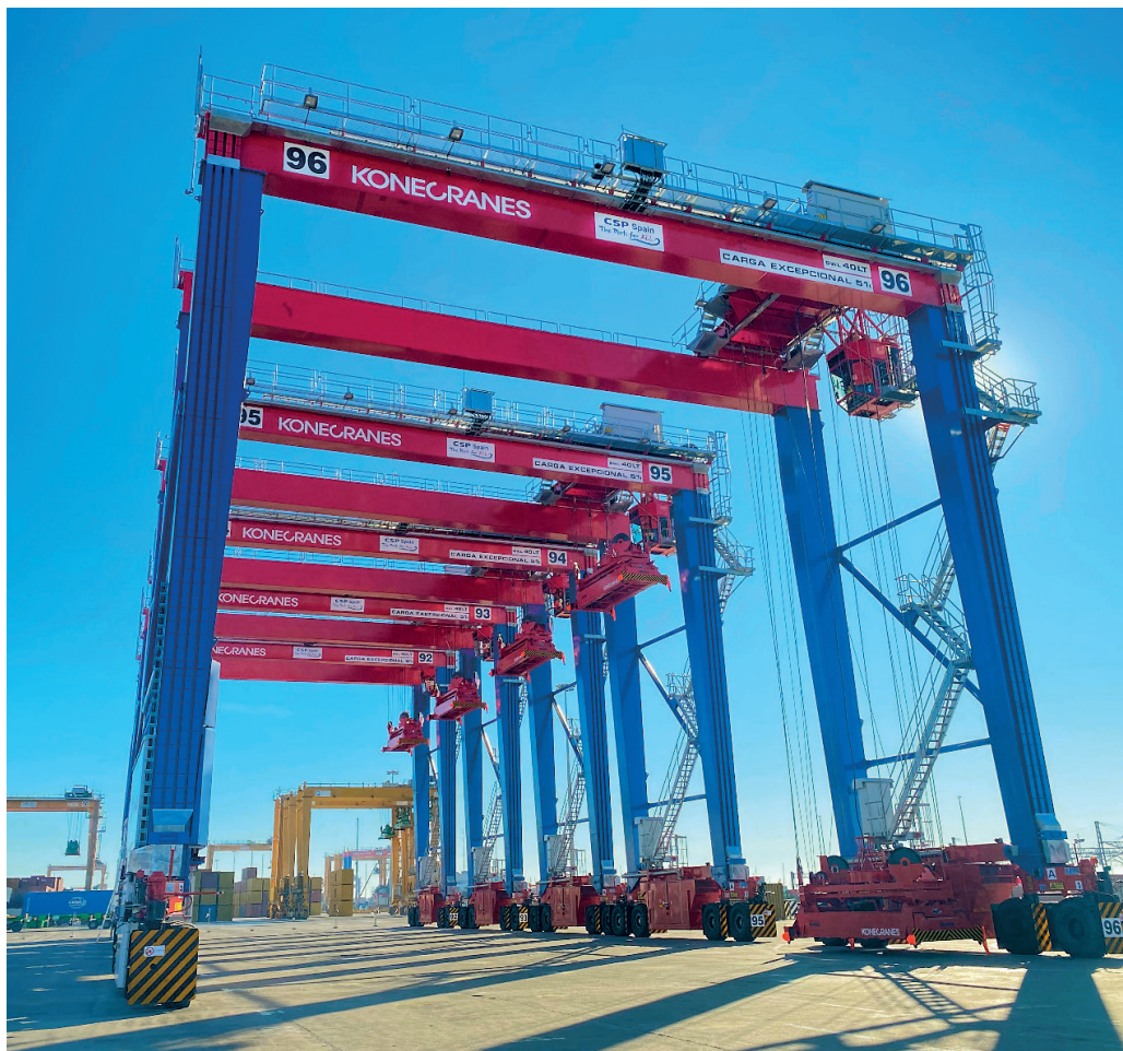
Konecranes ha invertido en tecnologías de retrofit como los sistemas híbridos y electrificados para grúas RTG (rubber-tired gantry cranes). / Konecranes has invested in retrofit technologies such as hybrid and electrified systems for rubber-tired gantry cranes (RTG).
